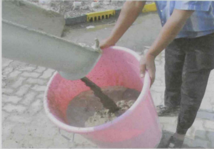
Figure 9: Wash water generated from concrete truck drum
